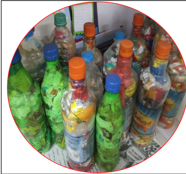
Creation of plastic bottle bricks and demonstration shown by students.
