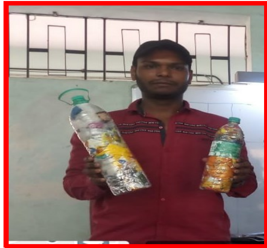
Creation of plastic bottle bricks and demonstration shown by students.
